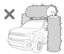
Racks must be removed when vehicle is put through an automatic car wash.
