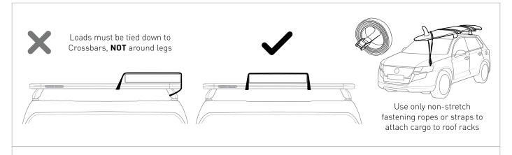
Tub/tray/canopys can move independently from the vehicle cabin. Rigidly fix to either the cabin roof racks **or** the tub/tray/canopy roof racks but not both simultaneously.
