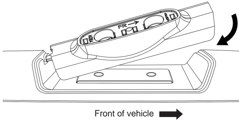
Position the Pad so that it sits flush in relation to the rail moulding.
