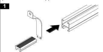
Place the conduit pipe onto the rubber strip.
