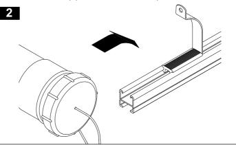
Slide the outer pipe clamp into the crossbar, slide the inner and outer clamp together around the conduit pipe.
