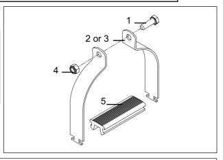
Slide the inner pipe clamp into the top section of the Rhino crossbar. Insert the rubber strip into the Rhino crossbar at the position where the conduit pipe is to be located.
