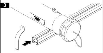
Insert the M8 x 25mm bolt through the pipe clamps, screw on the M8 nyloc nut and tighten to secure the conduit pipe. Do not over tighten the clamps, as this will crush the conduit pipe. Check that the conduit pipe is secure and cannot move on the crossbar.
