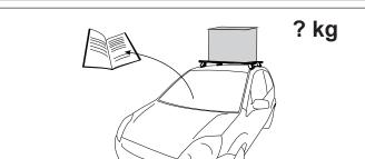
When these roof racks are to be used on a vehicle that is driven off sealed roads, the manufacturer maximum roof load rating (to be found in the vehicles User Manual) should be *halved*. Do not forget to subtract 7.5kg from your maximum carrying capacity due to the weight of the crossbars and legs.
