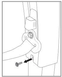
Unclip the seat belt cover using the clips at the back, then unscrew the nut using a 14mm socket wrench.
