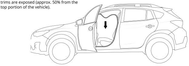
Move the seat back and recline for best access (don't do this if the seats are powered). Use thin forked trim tool to undo 2x clips behind the lower b-pillar and gently pull it away from the wall enough to access to upper b-pillar screw and unscrew it with a phillips head screw driver or 10mm socket wrench.
