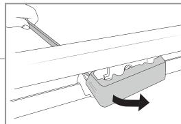
Clips holding cover in place are located on each side (interior surface).
